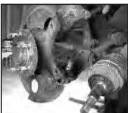
Free up the knuckle assembly...
